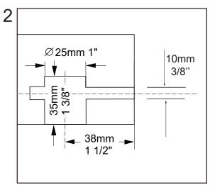
Mark and bore 1" (25mm) hole first then bore 3%" (10mm) hole.
