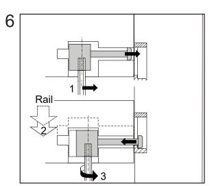
The shaft should be flush or under the surface of the end rail. Using a 5mm hex bit in a hand tool insert into gear housing, now it is possible to move the shaft to engage the disc keyhole. Then simply push rail downwards and tighten. Plug hole and sand.
