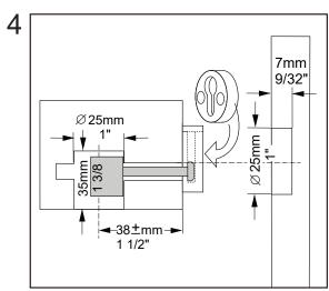
Insert connector into rail, check travel left to right.
