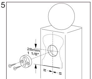
To mark the centre of the keyhole disc measure 1 1/8" (28mm) upwards from the bottom of the rail position. Using a 1" (25mm) bit bore hole into post 32" (7mm) deep so the keyhole disc is flush or slightly under. Secure disc with screws, bore pilot holes first.
