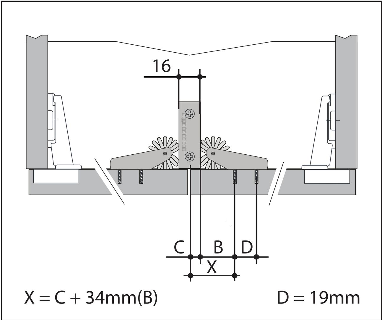
Daisy Catch Inline can be used against the Easy Cleat surface or directly against an end panel
