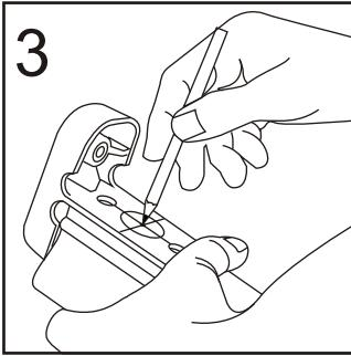
Using a pencil, mark the spot where the 1" hole on the bottom of rail will be drilled. **IMPORTANT!** **Drill the 1" hole first before you drill the 3/8" hole.** If not, it is possible that the bit will wobble and create imperfect hole that the 1" bung will not fit properly.
