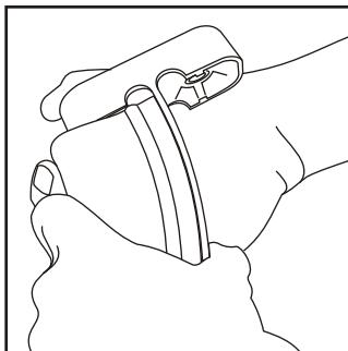
The jig can also be used with an easement. Mark centerline, press firmly into end. Holding the end with one hand and aligning the flap bending it to fit the easement align the holes through the windows in jig. Once lined up, the flap can be released and hole can be drilled. The "positioning pins" will help hold it in proper position to drill hole.
