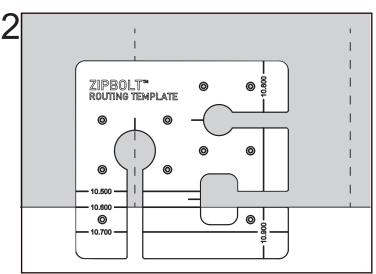
Once the Zipbolt model is chosen, select the appropriate marked line on the template and place over the edge of the top/panel. Make sure the template mark meets squared lines.
