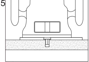
Set finished depth on router plunge, however, routing in two steps is recommended.
