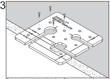
Secure template using 4 or 5 screws.
