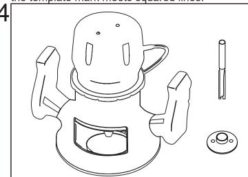
Tools needed: Router, 5/8 diameter short nose bushing and 3/8 diameter, long shank router cutter.
