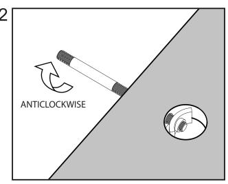
Place curved end plate into 1" (25mm) hole and engage screw shaft turning anticlockwise.
