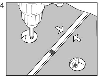
Use 4mm hex bit in power tool on low torque setting to tighten the connector
