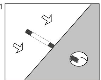
Pass screw shaft through edge of board.
